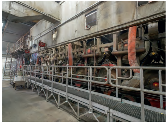
Drying section of PM1, reconfigured by AJ to eliminate one dryer fabric (see main article)
